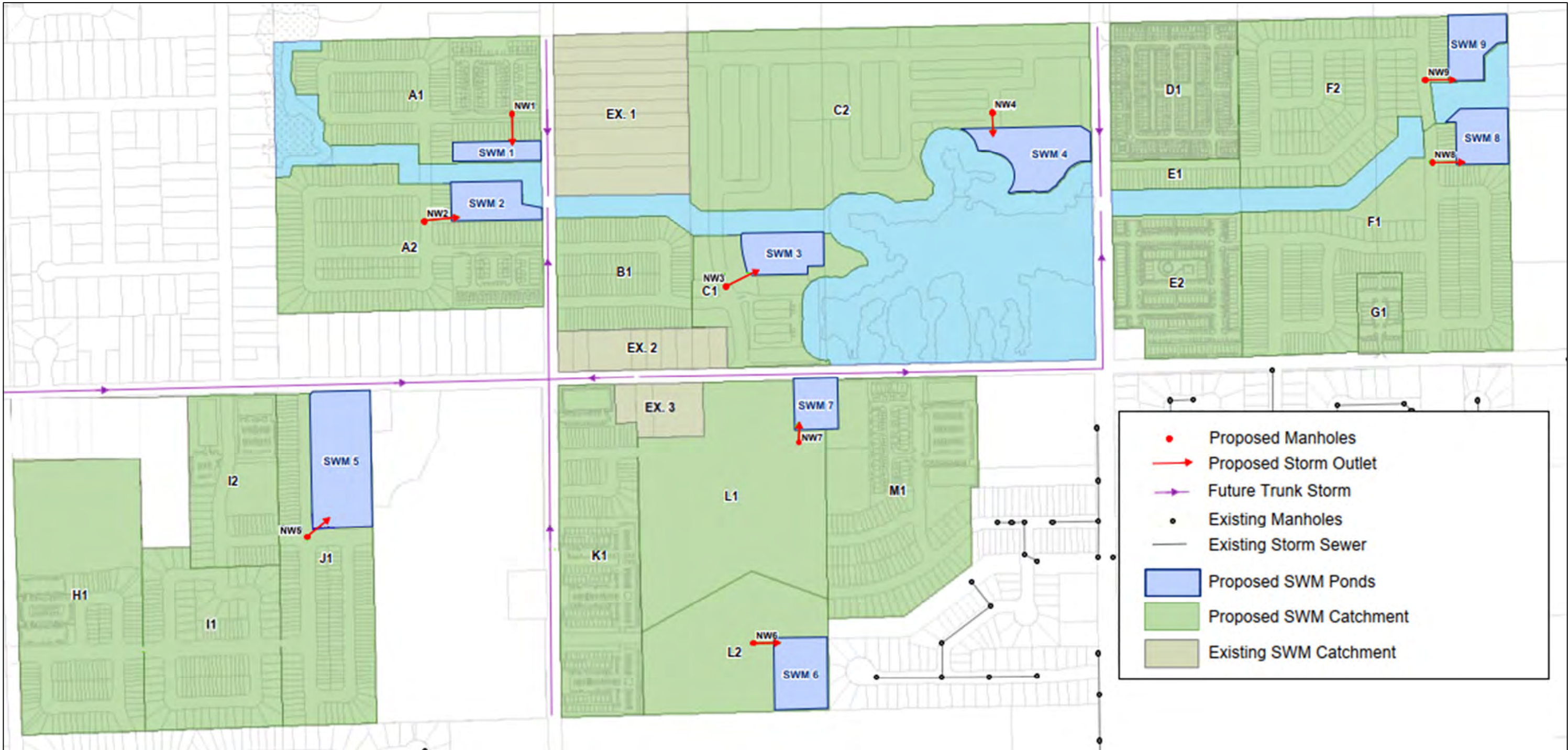
Figure 5-2: Proposed Storm System and Drainage Areas
